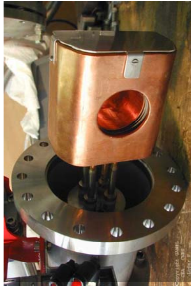
Figure 2: A 6-kW water-cooled Faraday cup in operation at GANIL.
