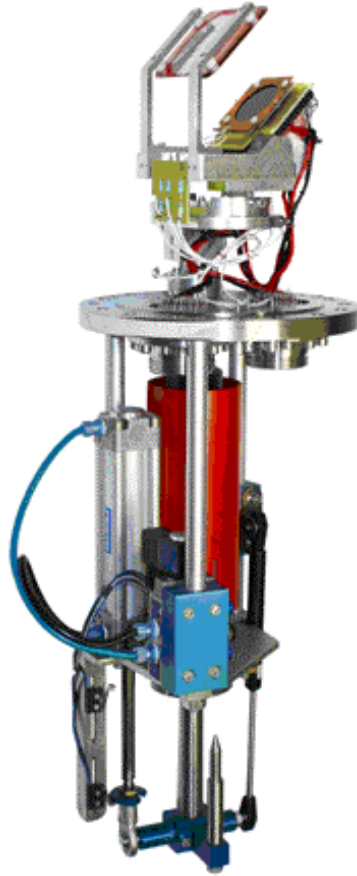
Figure 7: General view of the prototype of the secondary-emission beam profile monitor (equipped with a multi-channel plate) under development and test at GANIL.
